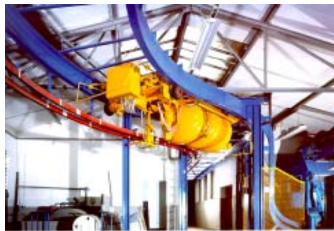
Feed and control of a concrete skipper
